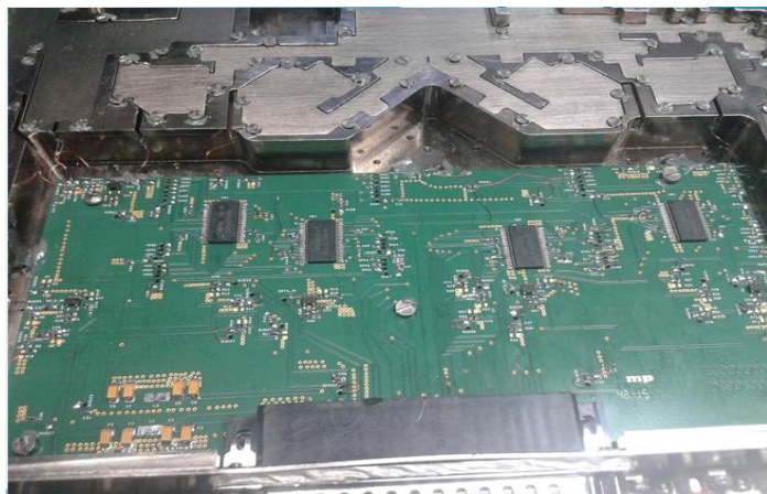
Fig-9. Power Supply & Control Distribution section
